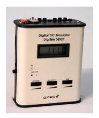
For T/C simulation, the output is cold-junction compensated according to the characteristics of the simulated T/C. In the **Measurement** mode, mV or temperature of the connected T/C can be directly read on the display.
